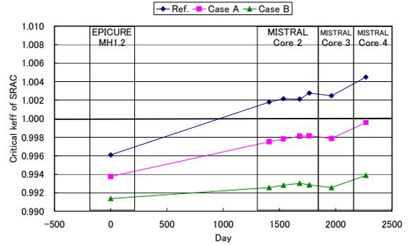
Figure 2 Critical keff of with increase of <sup>241</sup>Am capture cross section[8]
